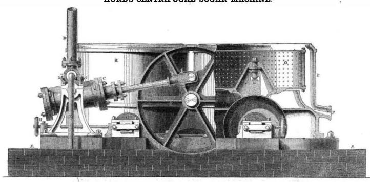
The accompanying engraving is an elevation partly in section of this sugar depurating machine, exhibiting the manner in which it is driven, and the machinery employed forthat purpose. Let us first present the description.
