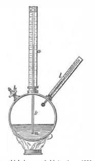
grees; this is now assumed to be about the latent heat of steam. A cubic inch of water, raised into steam, will, if confined in a tight vessel, and 5½ cubic inches of water, at 320, injected into it, raise the whole of that quantity to 64 cubic inches of water at 2120-that is, the steam will be condensed into water, and the cold water elevated 1800 in temperature; this experiment proves the theory of latent
