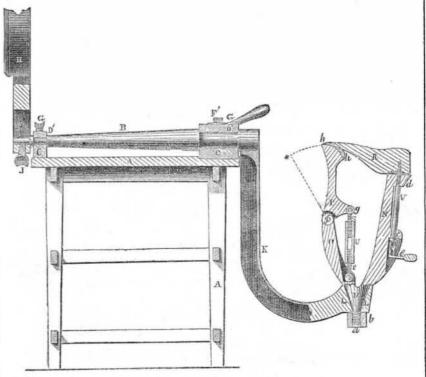
This engraving is a vertical longitudinal sec- | and retain it firmly in its position, until it is tion of the Revolving Last Holder, invented by Henry G. Dewitt, of Napanock, Ulster Co., N. Y., and for which a patent was granted on the 9th of June last (1852).
