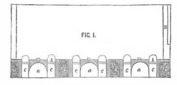
This invention is an improvement in the causing a free, steady, and unimpeded heat construction of Brick Kilns for burning coal equalized throughout the body of the kiln, or hard wood, and was patented by the in- by which fuel is economized and the time ventor, William Linton, of Baltimore, Md., required for burning the kiln shortened.
