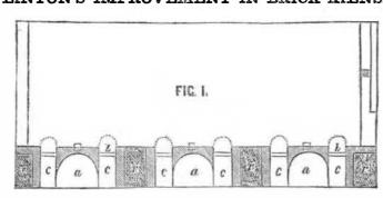
or hard wood, and was patented by the in- by which fuel is economized and the time ventor, William Linton, of Baltimore, Md., required for burning the kiln shortened. on the 20th of last January, 1852. The improvement consists in the form of the air ber, as situated a little below and between and in the mode of introducing the air into view of the kiln, with a portion of the wall the kiln for igniting and burning the fuel, and removed to show the fire beds. Fig. 3 is a
