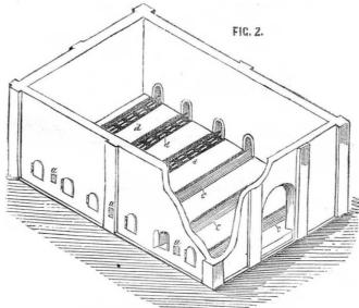
sectional view of the air chamber, showing air to every portion of the fire beds, for the the openings or recesses.
