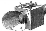
The accompanying engravings are views of G, of the chamber, B. F is a handle to throw trander, of this city, and patented on the 4th within each mouth of the tube of an alarm close the mouth when not in use, so that currents of air are prevented from passing through, and the other is to afford a signal by a sharp whistle, to direct the attention of those who may be distant from the tube when signalled
