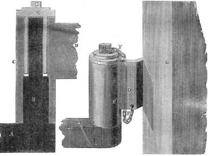
The accompanying engravings are views of | building-or only half way a most valuable improvement in Blind and part open. Shutter Fasteners, which was patented on the 11th May, instant, by Samuel Barker, of this lows:-The upper portion of the pintel of the
