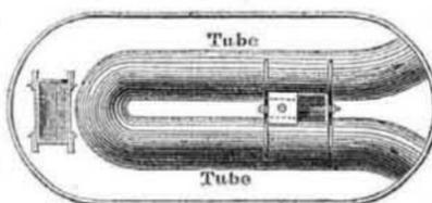
current. In a boiler the water is always agitated, but it is prevented from boiling in the inside of this sediment vessel, consequently the more violent the water boils in the boiler, the more rapidly is the sediment collected. For calcareous incrustations, this sediment collec-
