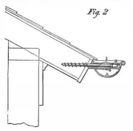
not injure the shingles, and is easier to adjust in its place. Any kind of metal may be used in constructing the gutter, or any modification of shape desired, to correspond with the architecture of the edifice, can be given it.
