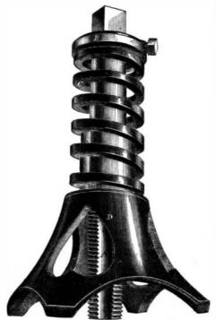
quite an original idea, nothing of the kind ever have ing come under our notice before. We have, however, often seen the want of such an apparatus, and can cheerfully recommend it as being a very useful tool. It is very light and simple in its action. A cast-iron stand, D, having a hole through its center to admit the tap, A, is provided with spring, C, and bland, cream jelly.—Exchange.
