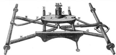
improvement in Hanging Carriage Bodies, which is bolted to the body, having on its back which was patented on the 22nd day of last or inside sockets fitting on the cross bars, E E. July, by the inventor. Mr. John Jones, of The guard-iron and step form a part of this Clyde, Wayne Co., N. Y., the inventor of the casting. The centre of the bars, E E, and the machine which printed the letter on page 166, joints where the stays, F F, are attached to the
