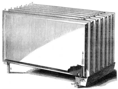
tive view, with a small portion of the shell removed, of the apparatus of Mr. A. S. Lyman, of this city, for heating apartments by steam, and for an exterior condenser tor steam en-
