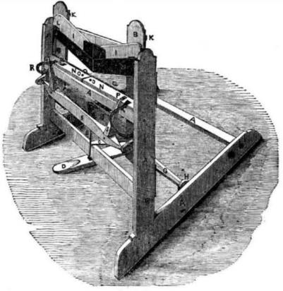
tive view of the improved stave jointing ma- the lower steel knives, Q Q, are secured by chine of Mr. Daniel Drawbaugh, of Cedar Springs, (White Hill P. O.,) Cumberland Co., the upper sides of the pieces, N N. Near each Pa., and which was patented on the 11th of outer end of the adjustable pieces, N N, there
