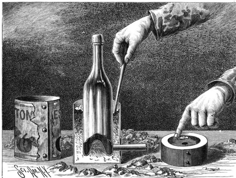
FIG. 11.—MAKING A BLOWPIPE FURNACE.
