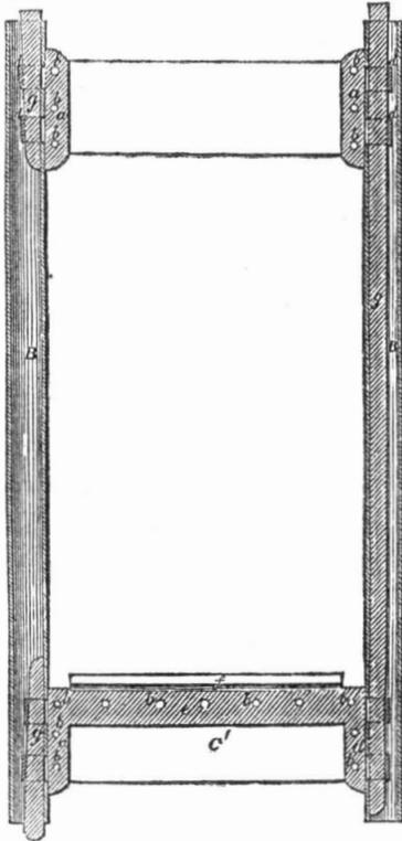
The improvements consist in the construction of the frames, whereby great strength is combined with lightness, and it can be easily taken to pieces and put together so as to render it portable. A false frame is also provided,
