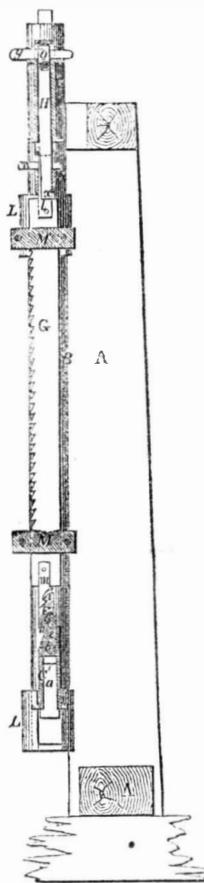
The accompanying engravings represent improvements in Saw Frames, invented by Mr. William C. Bronson, of Erwin, Steuben Co., N. Y., who has taken measures to secure a patent for the same. Figure 1 is a front elevation of part of a saw mill; figure 2 is a vertical section, taken transversely to figure 1. Figure 3 is a vertical section of the saw frame. Figure 4 is a horizontal section of the saw frame taken at the top. The same letters refer to like parts.
