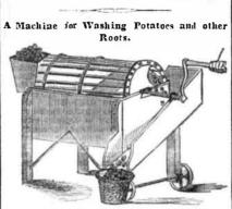
This is an Archimedean potatoe washer. The roots to be washed are placed in the cylinder at the farthest end from the crank, the cylinder being partly immersed in water. By turning the handle in one direction the roots are washed; and when sufficiently cleaned, by turning it in the contrary direction, the Archimedean screw inside the cylinderinstantly empties out the contents, as shown in the illustration.
