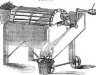
This is an Archimedean potatoe washer. The roots to be washed are placed in the cylinder at the farthest end from the crank, the cylinder being partly immersed in water. By turning the handle in one direction the roots are washed; and when sufficiently cleaned, by turning it in the contrary direction, the Archimedean screw inside the cylinderinstantly empties out the contents, as shown in the
