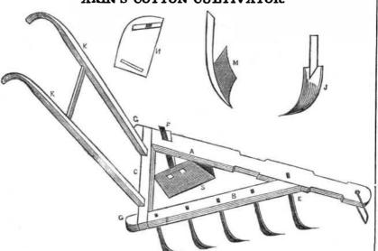
This Cotton Cultivator is the invention of | angling beam, B, the fore tooth through both Mr. Sam. W. Akin, of Spring Hill, Maury Co., beams A and B at E, set at equal distances Tenn., and secured to him by patent on the 20th apart, two feet two inches to the hind tooth of March last year. A, is a beam 4 feet long, longer in proportion for rows over three feet teeth; the fore tooth 15 inches long, falling
