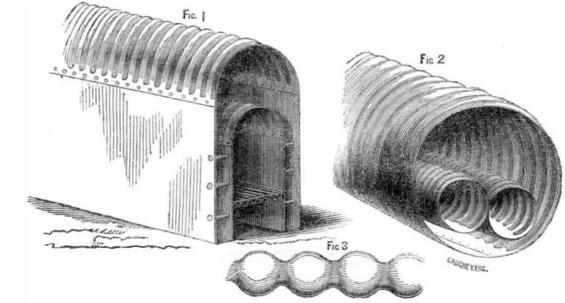
tops of flues, and the bottoms of cylindrical boilers, a great extension of effective heating surface is obtained, consequently the sufficient steam generating surface may be had in a reduced space without any increase in the weight of the metal. Experiments have proved that the corrugated boiler plate, in an arched form, with the flutings running in the direction of the arch, possesses such great strength that it
