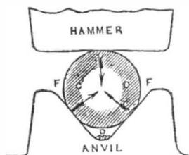
surface of junction it occupies. The frequency of this interposing scoria as the true cause of unsound forged work, was forcibly alluded to by Mr. Nasmyth, and shown to be the most fertile source and cause of the failure of wrought iron work, resulting as such too frequently does in the most sad and disastrous accidents—such as the failure of the links of chains and anchors, and in the costly and often distressing results arising from defective (i.e., blistered) boiler-plates.
