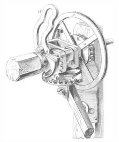
pinion, K, having an equal number of teeth, which causes it to revolve once on its own axis during each of its revolutions around the shaft of the reel. This imparts such motion to the crank on the end of the axle of pinion, I, as to bring this crank to the lower end of the slot in the arm, H, just as the rake has completed its passage across the platform, and then this crank, in its onward movement, carries the collar, C, and with it the rake, around the shaft of the reel.
