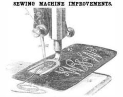
We herewith illustrate further improvements added to the Wheeler & Wilson sewing machine, namely, the "braider," a device for sewing braid or cord upon any kind of fabric. The braid or cord is passed through the hole, 72 (see engraving), of the ordinary glass presser, 71, of the machine and stitched upon the fabric, 46, in the most elaborate designs without any previous basting. Its value is best set forth by a lady's hand as follows :-
