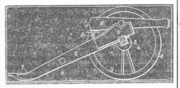
cheeks, 2, the axle tree, 3, the wheels, 4, and the elevating screw, 5.
