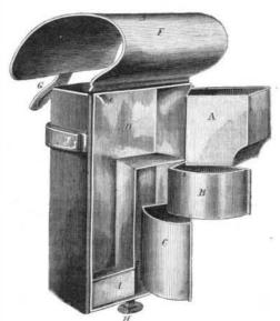
The lowest drawer of the box may contain a vial of oil and a pin for cleaning the tube. These are held by an open ring which is soldered to the inside of the drawer in such a manner as to form a spring to hold the vial and pin without breaking, and still to allow a larger or smaller vial to be used.
