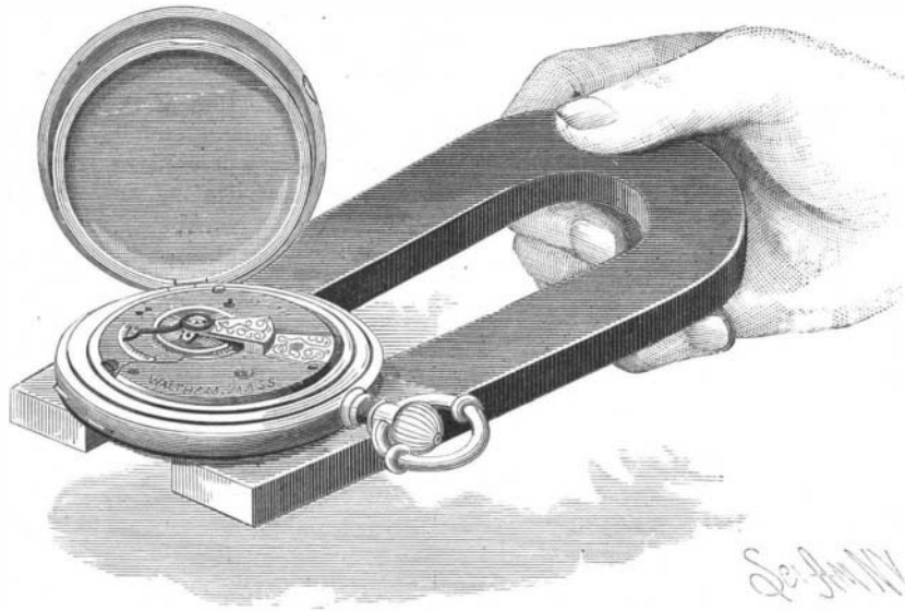
TESTING WALTHAM WATCHES WITH A HORSESHOE MAGNET.
