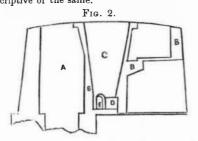
Fig. 1 represents an elevation of the usual formin which kilns to burn lime with coal are frequently built. A is the front wall of the kiln; B, part of a slope made to enable the workmen to mount up to the top of the kiln, to charge it with coal and lime-stone, in alternate beds. C one of the three arches that lead to the fire-room, and through which the lime is withdrawn.
