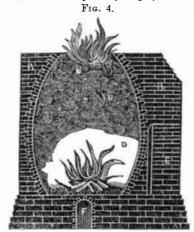
drops it into the fire-room, and immediately stops up the fire-room door with another fagot and so keeps on : F, the arch-room, which is an arched vault that crosses the bottoms of the kiln; it has a hole in its middle which corresponds with the fire-room, and lets the small coal pass into the ash-vault.
