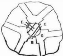
Fig. 3 represents the plan of the kiln. E the three arches leading to the fire-room; O iron bars placed across the bottom of the fire-room, to serve as a grate and supporter of the lime-stone.
