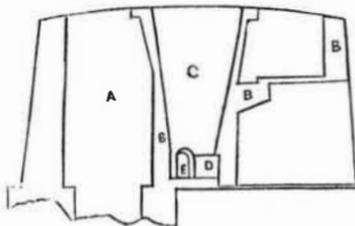
Fig. 1 represents an elevation of the usual form in which kilns to burn lime with coal are frequently built. A is the front wall of the kiln; B, part of a slope made to enable the workmen to mount up to the top of the kiln, to charge it with coal and lime-stone, in alternate beds. C one of the three arches that lead to the fire-room, and through which the lime is withdrawn.
