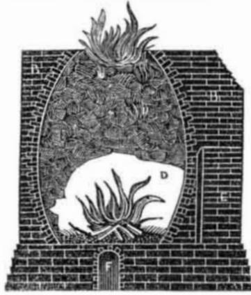
drops it into the fire-room, and immediately stops up the fire-room door with another fagot and so keeps on: F, the arch-room, which is an arched vault that crosses the bottoms of the kiln; it has a hole in its middle which corresponds with the fire-room, and lets the small coal pass into the ash-vault.
