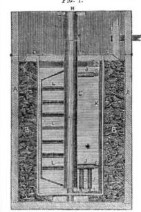
This is an Ice Cream Freezer, invented and patented by Mr. H, B. Masser, Editor of the Sunbury American, Pa. Figure 1 is a vertical section, and figure 2 is a section of the scra-
