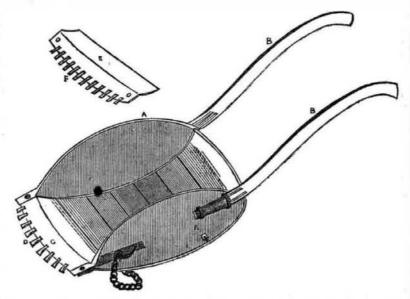
has a patent for the improvement. The disface, the teeth being in condition and number adapted to the condition of the soil in which B B are the stilts or arms, C is the moveable those who have used it. mouth piece with the teeth D. The teeth on the mouth piece of the excavator, are broad gravelly soil : the teeth, F, in the detached teeth. mouth piece E, are narrower at the extremities and are adapted to excavating in stiff and addressed to Mr. Sweet.
