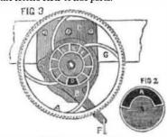
LLLL is the frame; P is the grain box. raised to show the distributors; O is a cranked shaped cast arm, bolted to the centre crossbeam of the frame; A A A are the seed wheels or distributors, which turn on plates bolted to the plates into the tubes.
