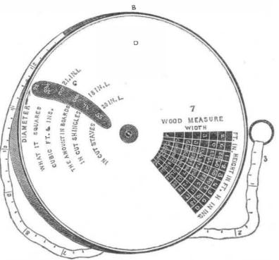
ar plates of brass, held together by an outer popposite the figures, on the plate C, at the side rim, through which is made to pass the tape of the opening therein, (which figures indiinto and from the wheel which is enclosed in- cate the length of the board from 7 to 19 feet) side. The tape is marked out into 48 inches.
