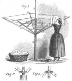
the arms, c c. Braces, d d, extend from near the middle of the arms, c c, to a second collar surrounding the shaft, b, represented in Fig. 2. Lines, e e, connect the two collars, and by tightening these lines so as to draw the two collars together, the arms, c e, are pressed outward, and the lines connecting them are stretched taut.
