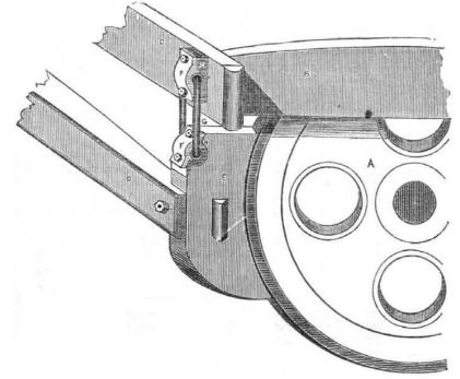
made with another box similar to the one described, both lettered alike, which encloses the other end of the link, G, thereby enabling the brake to be applied so as to adapt itself to cause the brake to be applied at all times to the wheel at all times, with the same force, through the whole arc of the brake, and not more at the top than at the bottom.
