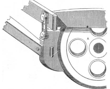
made with another box similar to the one described, both lettered alike, which encloses the other end of the link, G, thereby enabling the brake to be applied so as to adapt itself to the wheel at all times, with the same force, through the whole arc of the brake, and not more at the top than at the bottom.
