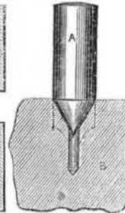
In some instances, the old forms evidenced a less amount of friction than the new one, but this was for a limited period only at the commencement, as very quickly the destructive wear, increasing towards the centre, caused so much friction that the parts adhered firmly together.
