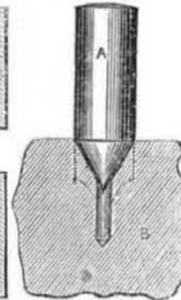
In some instances, the old forms evidenced a less amount of friction than the new one, but this was for a limited period only at the commencement, as very quickly the destructive wear, increasing towards the centre, caused so much friction that the parts adhered firmly together.
