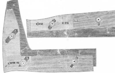
patented by him in the Provinces. Its object of any measured boot, and may be termed a "boot pattern guage." This engraving represents side views of the apparatus. Figure 1 is to measure and guage the leather for the back of the boot, and fig. 2 for the front; apparatus for the same purpose have been brought Railroad, payable in five years, were sold on forward before, but they were all defective in one
