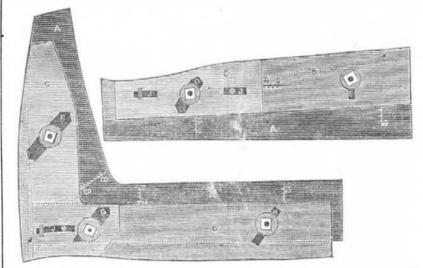
This apparatus is the invention of Mr. Jas. to guage the uppers uniformly, to fit them for patented by him in the Provinces. Its object of any measured boot, and may be termed a "boot pattern guage." This engraving represents side views of the apparatus. Figure 1 is to measure and guage the leather for the back of the boot, and fig. 2 for the front; apparatus for the same purpose have been brought
