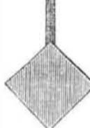
Lastly, the same blades were turned into the position of fig. 44, (being fig. 41 reversed.)—The boat was turned on No. 3 under all circumstances, describing circles from 80 to 150 feet in diameter. Four of them equalled eight of No. 3. They were thought to throw off more water behind than their competitors, which, from the greater extent of their extremities, was probably true.
