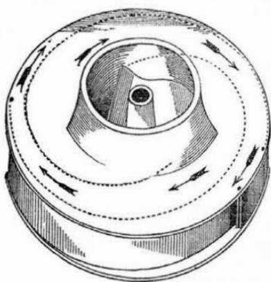
This is an engraving of T. R. Timby's Water Wheel. It is made with eccentric flanges, indicated by the dotted lines, and the arrows indicate the course of the water. This wheel receives the water at its centre, on a gradual curve, from a vertical to a horizontal. On this curve, the water is deflected so as to impinge with the greatest momentum, against two eccentric flanges, presenting surfaces gradually receding from the centre, and gradually diminishing in their eccentricity from the centre to
