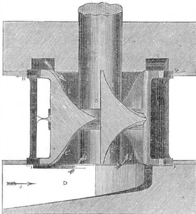
This improvement on Water Wheels is the invention of Mr. W. T. Collier, of Old Fort, McDowell Co., N. C. The wheel is a double acting submerged one, employing the re-active force of the water.
