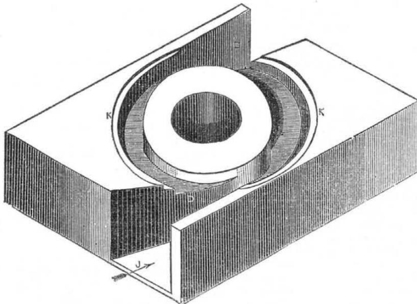
The wheel has two set of buckets, one above and one below, set at opposite angles but discharging in the same direction, and each set
