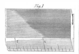
by the law of capillary attraction, absorb horizontally all ink that may descend from the edge along which the pen passes, a. The groove may, if preferable, serve the purpose of holding a narrow strip of blotting paper, which, extending and resting on the projection, c, will absorb the ink in its descent. The latter may appear the better arrangement to those unfamiliar with the action of capillary grooves, but the former will be found to be equally effectual.
