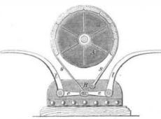
The construction and application of the brake will be readily understood by a glance at the above engraving, by which it will be seen that the brake consists of a drum. A. round which passes a strap or band. S S, having upon its under surface, where it comes into contact with the drum, stops of wood, or other suitable substance, for the purpose of causing great friction, and thereby effect the braking of the barrel which contains the chain working the rudder.
