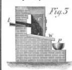
Fig. 3 is a very simple furnace employed for smelting the lead ore of the north of England and at the Scotch mines. C is a cavity of masonry lined with cast iron. The sole plate, s, is also cast iron, its back and sides are upright cast-iron
