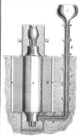
The mold, B, with the space, A, for the casting, is placed in a vertical position as usual, and round the outside of the mold is formed the annular space, C, to be filled with cast iron immediately before the casting of the cylinder. This heats the mold from the outside as well as from the inside, and thus prevents it from breaking. The metal is poured into the funnel, F, and passing through the vertical pipe, E E, and horizontal pipe, G, enters the mold by the lower journal, D.
