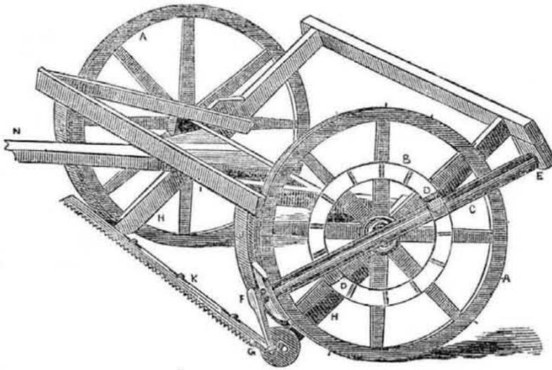
This machine is the invention of Mr. Homer Adkins, of Round Prairie, McDonough Co., Illinois, as noticed in our last number. It is made of two wheels, A A, like a cart, as shown in figure 1, which is a perspective view; and with reciprocating cutters, as shown in the section view, figure 2.
