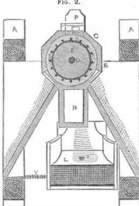
at the end with the outside and with the inside, driving the blast through the pipe, H, to cleanse the grain; I is the hopper, to receive
