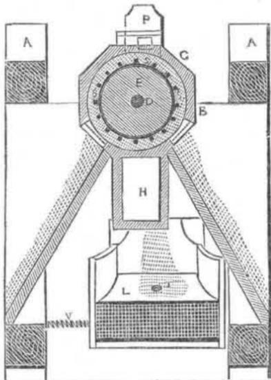
at the end with the outside and with the inside, driving the blast through the pipe, H, to cleanse the grain; I is the hopper, to receive
