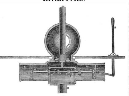
This pump is the invention of E. A. Jeffe- the uppermost parts of the barrels, hence any ry, of Corning, Steuben Co., N. Y., who has air which may have entered with the water made application for a patent. This is a ver through the suction pipe, will be first dischargtical longitudinal section, and exhibits all the ed from the barrel, and when the piston ar-
