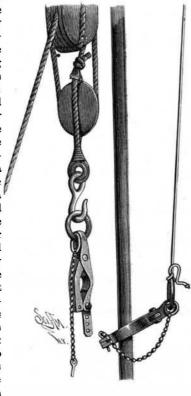
passed through without opening the jaws. In using the grapple two of them are necessary; one is attached to the pulley block for raising or lowering the pipe, and the other is suspended by a chain to some stationary beam, one or the other always being loose on the pipe. To use the grapple the pin is drawn from the one attached to the pulley, the grapple is opened, and the jaws passed around the pipe, when the pin is replaced.
