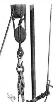
sume a right-angle position, allowing the coupling on the pipe to pass through freely. The stationary grapple holds the pipe while the other grapple is being shifted. The engraving represents one grapple attached to the pulley and the other in position on the pipe.
