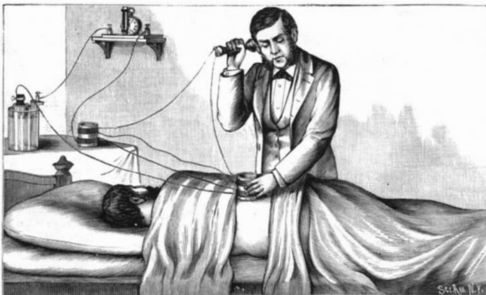
Fig. 1.—THE INDUCTION BALANCE USED AS A BULLET FINDER.
